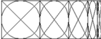
The solution is quite simple. But it's a boring repetitive task. You need to create the railing panel as a block, then insert it with different scale on one axis. See the complete explanation here.
